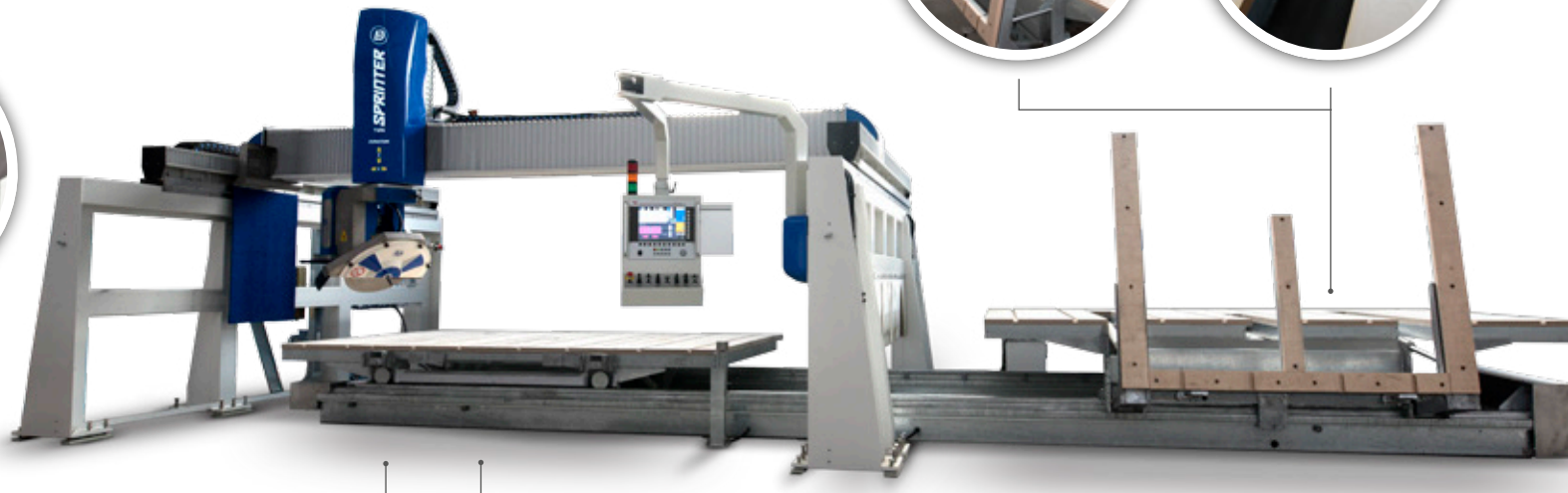
Monoblock steel structure to avoid concrete foundations below the floor level, on which the sliding rails of the benches are placed
