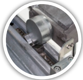
Wheels with locking system that avoids any micrometric displacement
